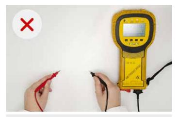
Wrong measurement (voltmeter with measuring tips)
