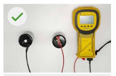
**Correct measurement II (with measuring probes)**
